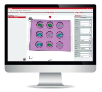
Improve your printing process definition, compose your print project by positioning your constructs precisely where needed on the print workzone, and define the printing material dispensing order.
