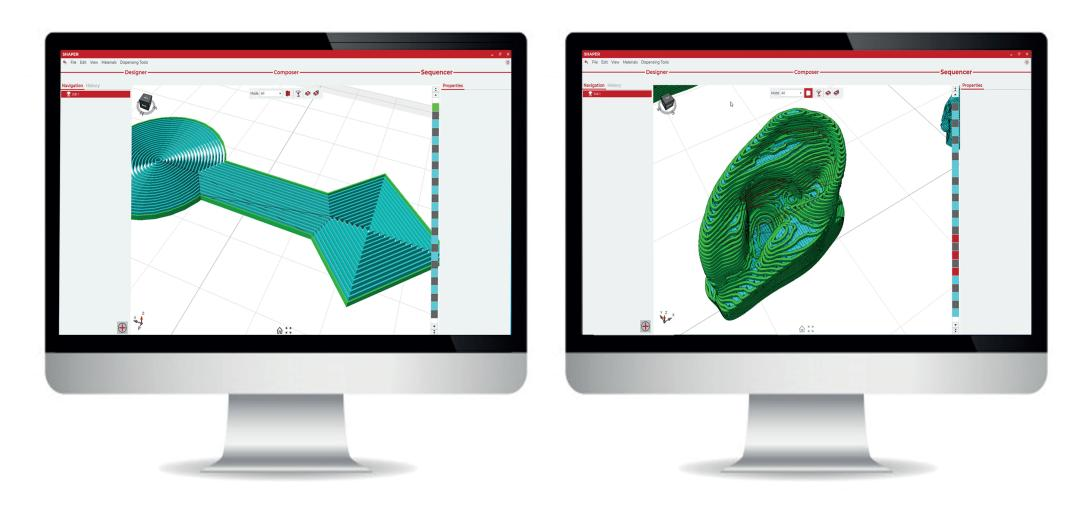
Use our powerful tools to easily design your 2D or 3D constructs, or import them from another source, define and select multiple printing technologies, and set parameters for the use of various biomaterials, in a single view.
